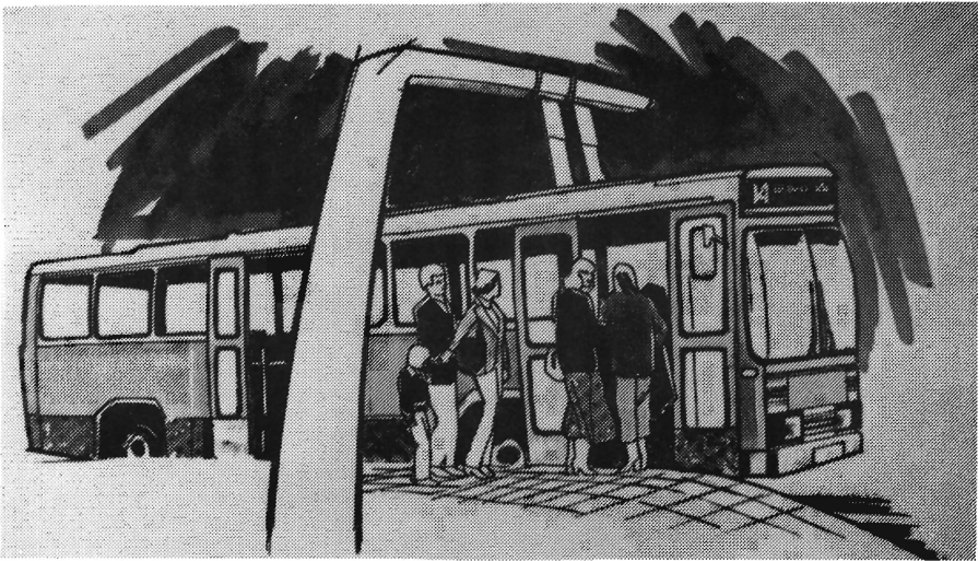
Photo 3.1. Charging of a fully flywheel driven city bus at the bus stop.
